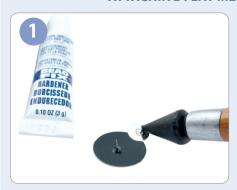
Place the focal component facedown on a flat surface and place a small drop of epoxy on the back of the focal. Press the slider component onto the glue. Let it dry.
